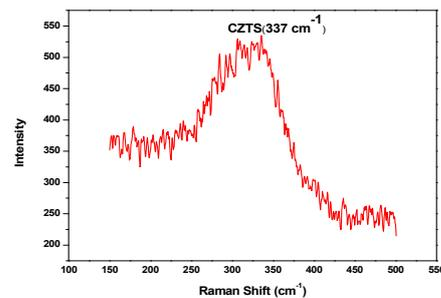
Fig. 4-Raman Spectrum(using Horiba Jobin Yvon
