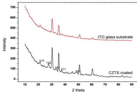
Fig. 3- XRD pattern of the CZTS film
