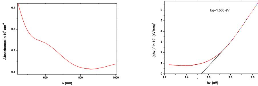
**Fig. 5-Uv-visible spectral data** (from Jasco V-570 Model uv-vis spectro photometer)
