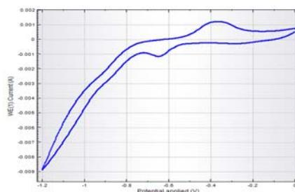
Fig. 2- Cyclic voltametry of the deposition process
