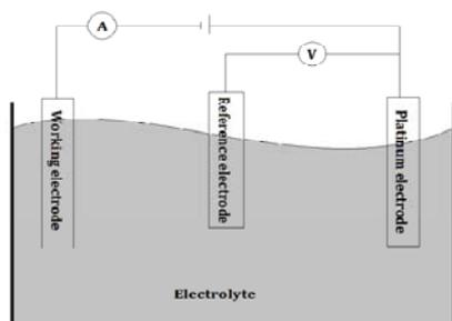
Fig. 1-Schematic diagram of the electro deposition system
